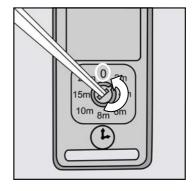
[2] Turn the switch time selector to the "0" position.
