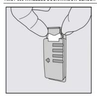
[1] Slide open the battery compartment and place a battery in the recess of the battery holder with the "+" pole face up. Now slide the holder back into the product.
