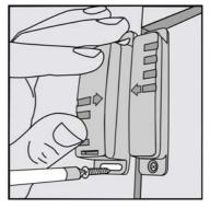
[6] Attach one of the parts to the door or window and the other to the frame. The arrows on the two parts must point toward each other. Attach the parts with as little space between them as possible.
